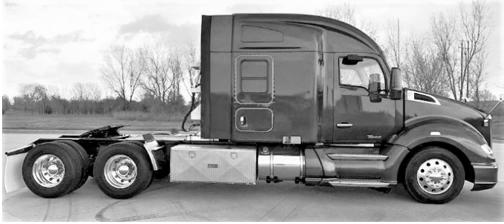
This is called a mid-roof sleeper and usually only has one bed in it.
