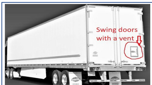
53ft dry van trailer with swing doors and a vent in the rear door which can be opened when needed.
