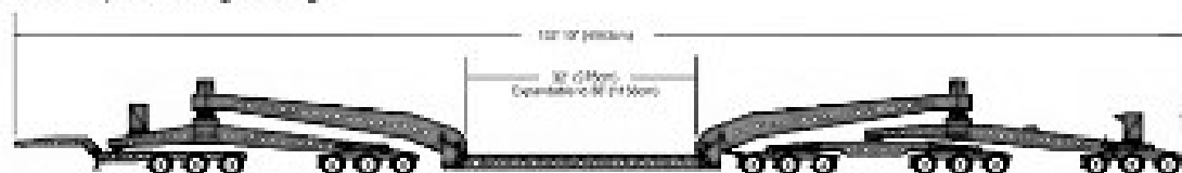
19 Axle Expandable High Tonnage
