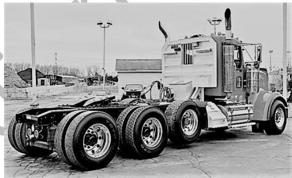
Day Cab Heavy Haul with tag axle raised
