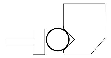
After releasing all compressed air from the tool. Confirm that the nozzle gripper clamp air cylinder is fully retracted. Loosen the cap screw bolt which holds the v-block gripper clamp on the rear side of the main plate & slide it as far to the right as possible. By having both the cylinder & V-block retracted, this will allow adjustment space for the positioning of the weld nozzle & reamer cutter.
