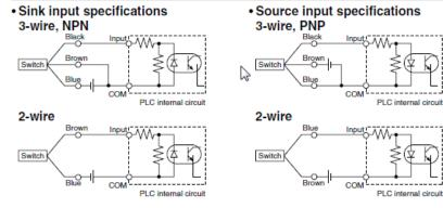
Connect according to the applicable PLC input specifications, as the connection method will vary depending on the PLC input specifications.
