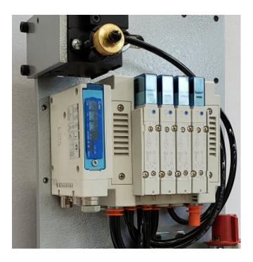
The SMC EX260 Fieldbus option is offered in a variety of common protocols listed below. Operations manuals, setup videos, configuration & EDS & IIOD files can be downloaded @ https://www.smcusa.com/help-support/instruction-manuals/fieldbus-products-ex-series/
