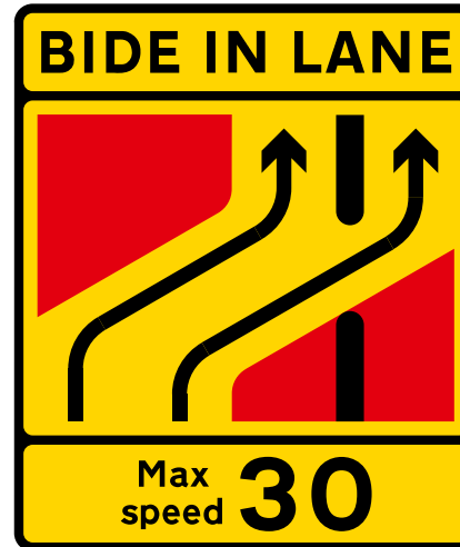
One lane crossover at contraflow road works
