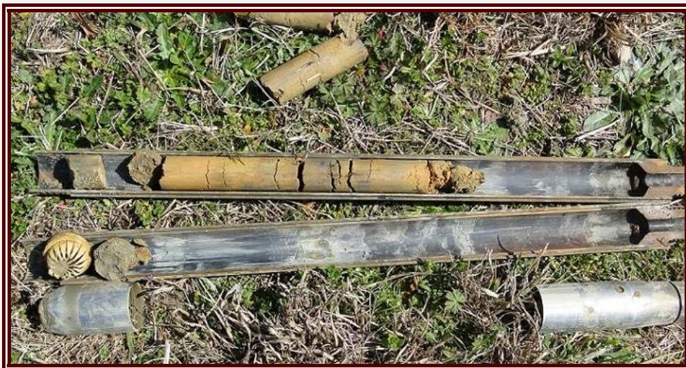
Figure 17 The split spoon sampler is a tube split into two equal halves lengthwise. The two halves are locked together during the sampling activities and released to retrieve the samples. At bottom end of the sampler sits a driving shoe. This is what cuts into the soil and provides the sample that goes up into the tube.
