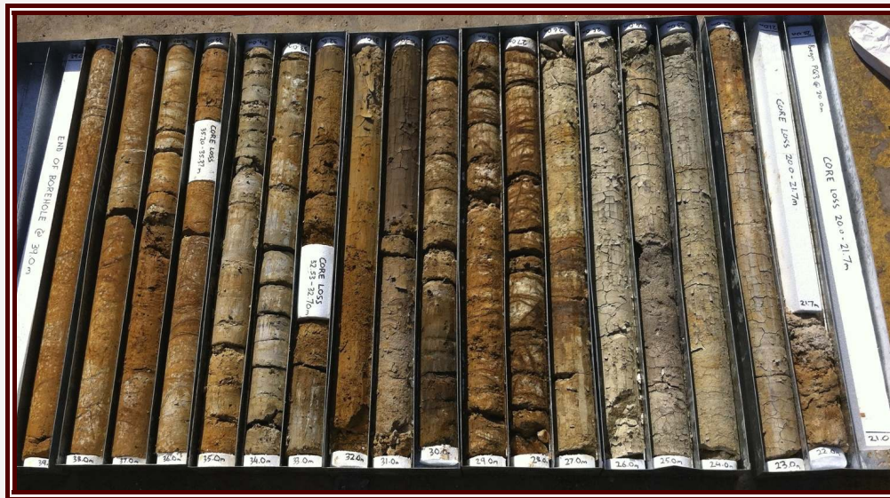
Figure 18 Soil cores from the ground within stratification layers from 1 st to 4 th Centuries. Scientists from the testing laboratory will determine radiocarbon dates for pieces of charcoal that came from ancient fire pits. A high frequency of charcoal will confirm a high density of habitation.
