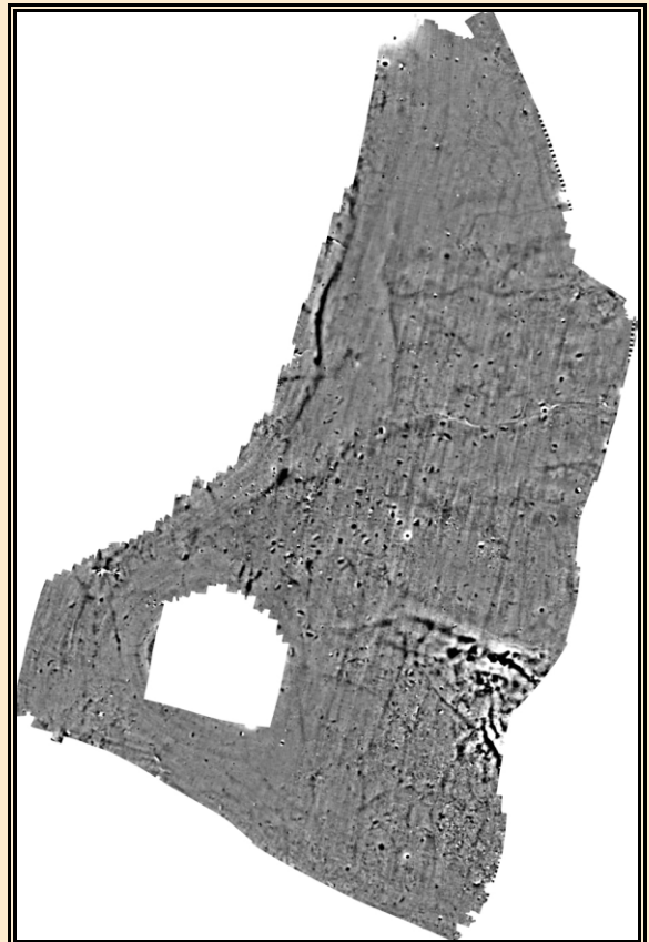
Figure 9. SENSYS December 2018 magnetometry scan of Fort Glenford hilltop field. The mound could not be scanned for obvious reasons but the array was pulled as close to the mound perimeter as possible.
