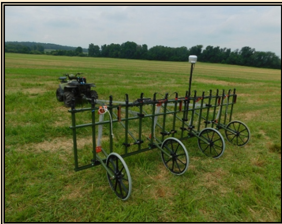
Figure 1. SENSYS MAGNETO ® MX V3. Large area magneto-meter survey system which has 16 fluxgate gradiometers arrayed on a trailer with a width of 3.85 meters.
