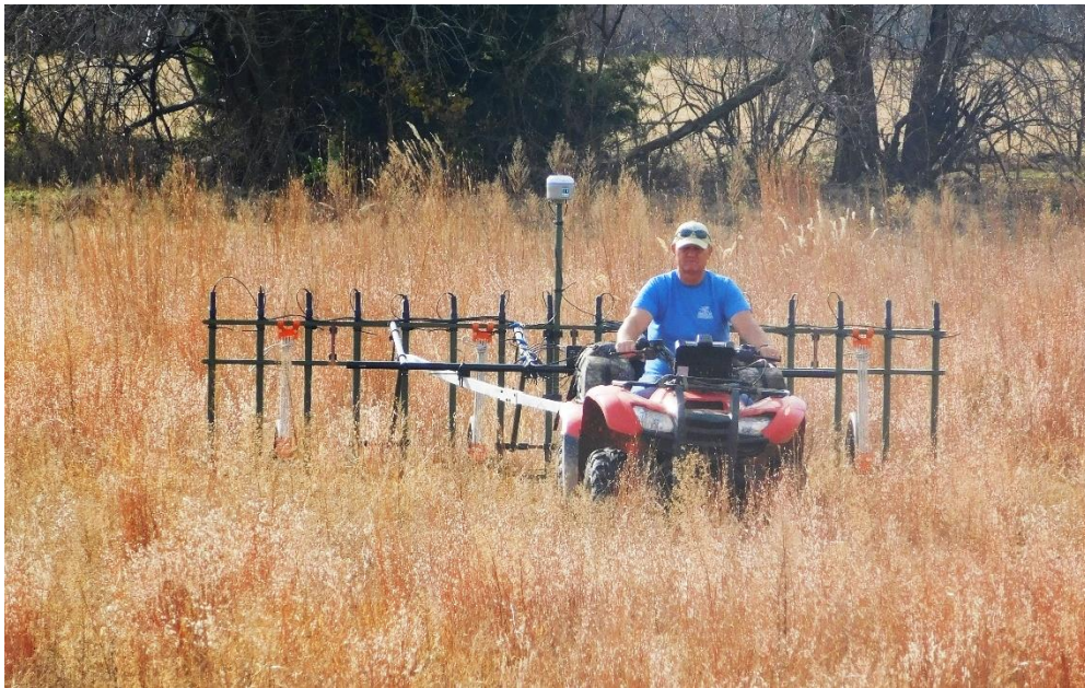
Figure 1. The 16-sensor array with the GPS responder atop the array.
