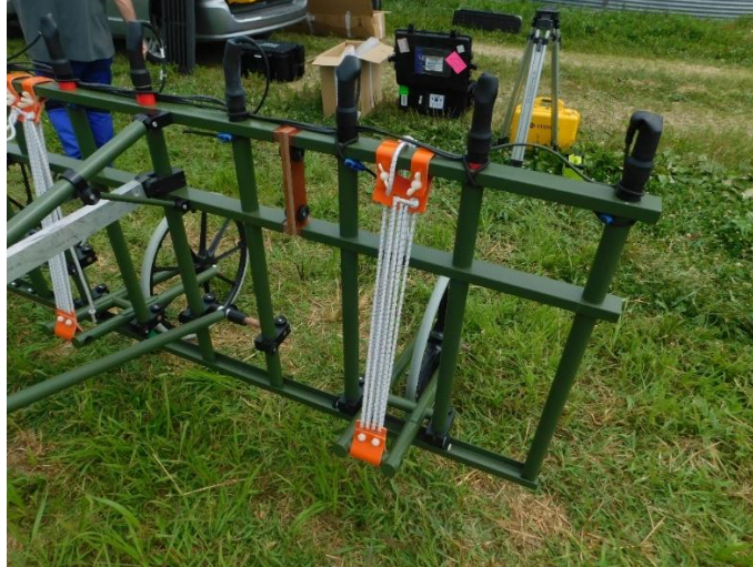
Figure 2. The shock absorption system of the device minimizes vertical oscillations.
