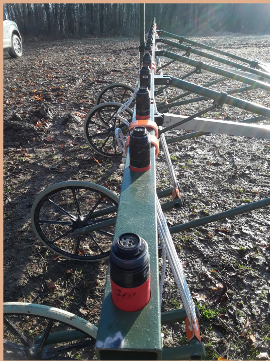
Figure 7 16 Magnetic Probes SENSYS MX Carrier Arrayed on 12.3-Foot Rack
