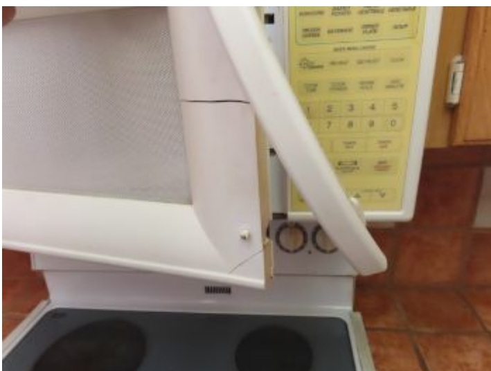
Damaged microwave door handle
