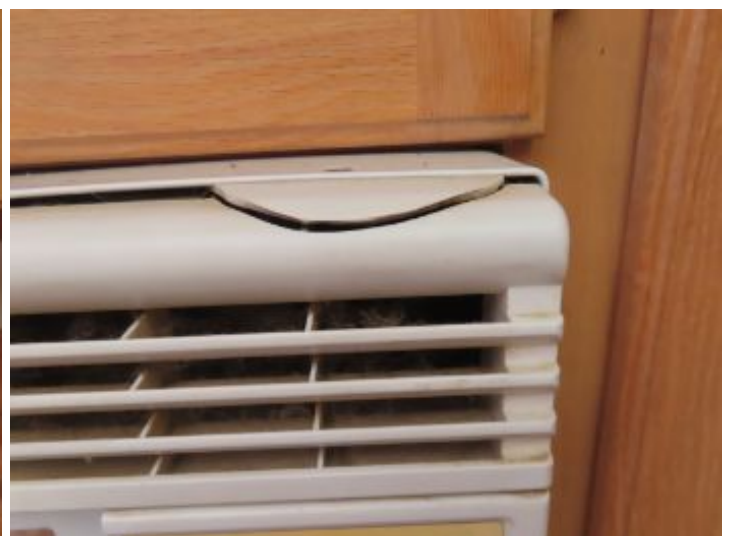
Damaged microwave housing
