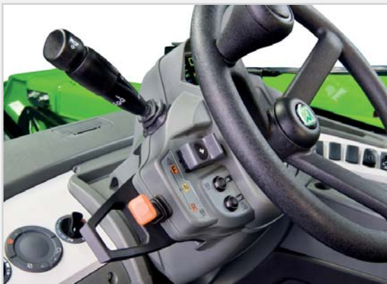
HM: dual-Shuttle reverse shuttle buttons
