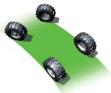
FRONT WHEEL STEERING MODE
