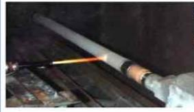
Coating of compressor rods for compressing gases or liquids in oilfields beingcoated with 86 - 10 - 4 tungsten carbide - cobalt chrome. It has a hardness of 1350 Vickers. After spraying it was ground to a mirror finish for less friction.
