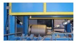
pistol traverses along the length of the bottle to coat the sides.
