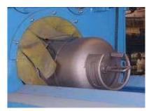
The surface of the bottles needs to be prepared to ensure an adequate profile is created for metal spray adhesion. This is done by grit blasting the bottles in an automatic blasting machine, which produces a blast cleanliness of SA 2.5. Once the surface has
