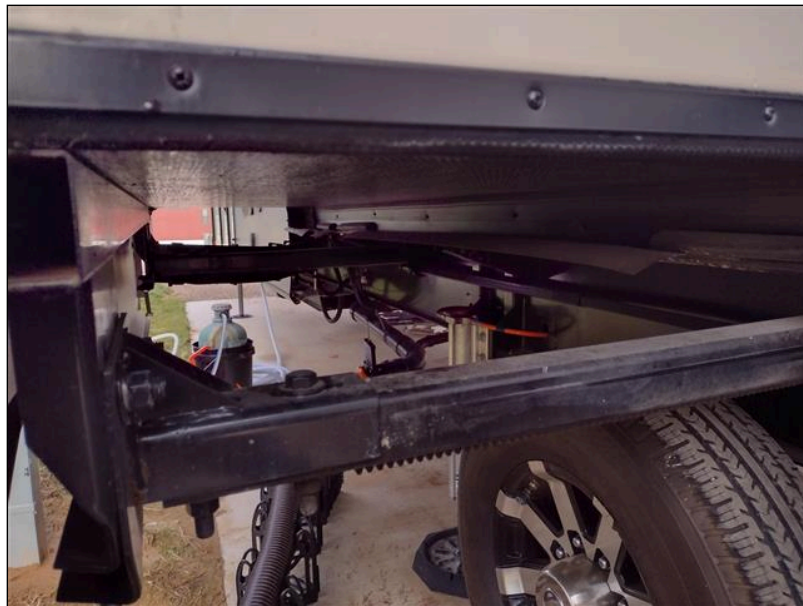
Hydraulic motor w/ Gear and rack system
