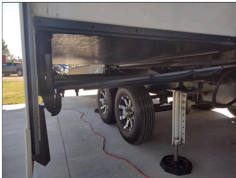
Hydraulic motor w/ Gear and rack system and wire harness.
