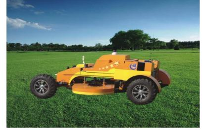
The mower is equipped with hybrid power, uses rechargeable batteries and automatically switches to conventional engine when additional power is required.
