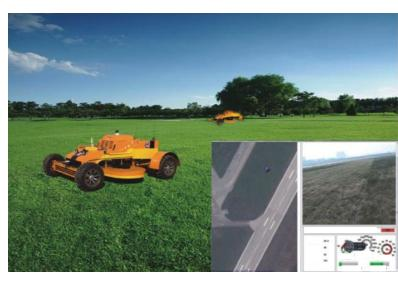
The remote monitoring station monitors the mower in real time, including live view of the vehicle accessible from both the web and mobile app.
