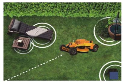
Combining obstacle avoidance sensor with GPS positioning system, the mower accurately identify roads ahead, avoid collisions, care for people, animal and its surroundings.
