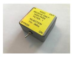
**HPF-1** (THE HPF-1 IS FOR RECEIVE ONLY, DO NOT ATTEMPT TO TRANSMIT THROUGH THIS DEVICE)
