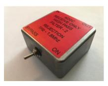
**HPF-2** (THE HPF-2 IS FOR RECEIVE ONLY, DO NOT ATTEMPT TO TRANSMIT THROUGH THIS DEVICE)
