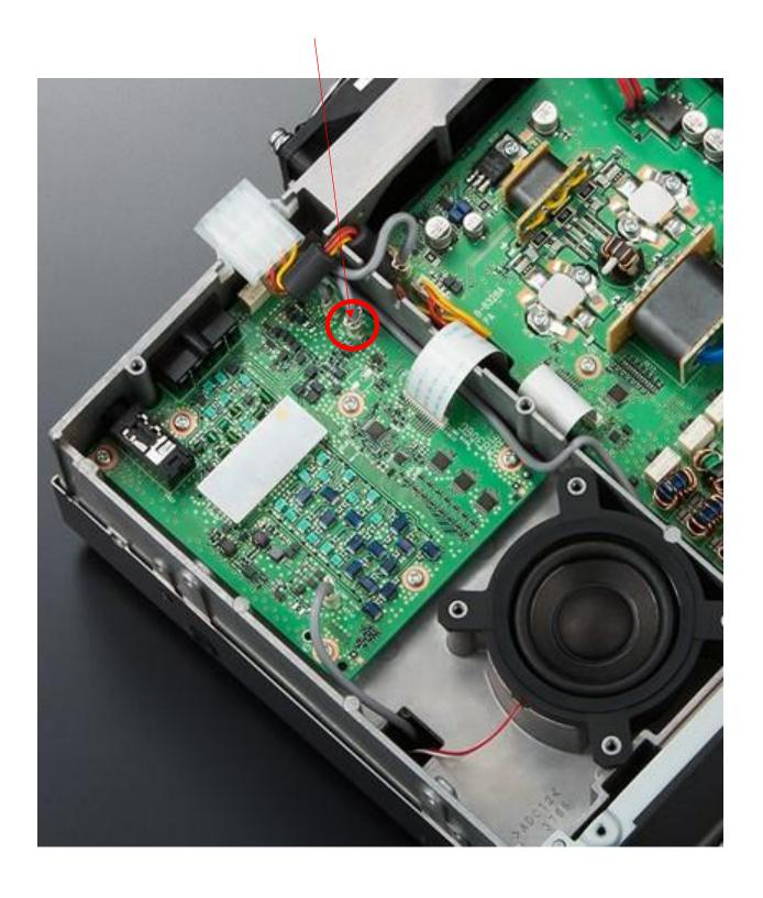
6. Lift and slide the Molex connector up and out of the slot. Fold it inward, connect the supplied Molex cable and connect the 2 pin power connector to (J4) on the PAT V 7300 board. Fold the supplied Molex cable and place wires outside the open slot left from removing the 7300 Molex connector.
