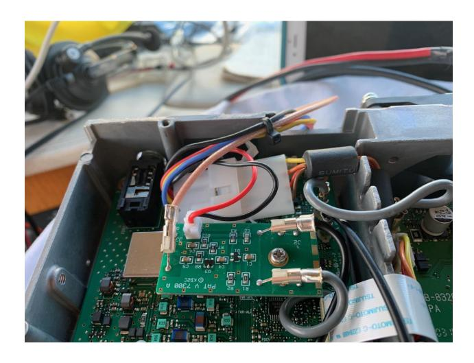
5. Unplug the Gray TMP cable from (RX) J1071 and plug it into J1 on the PAT V 7300 board. Plug the supplied Black TMP into J2 on the PAT V 7300. Plug the other end into (RX) J1071.
