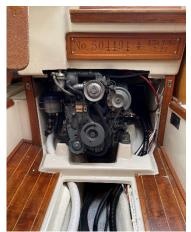
Vessel auxiliary power is by a Yanmar 2GMF, #10918 which was not run due to the boat being on the hard at the time of the inspection.
