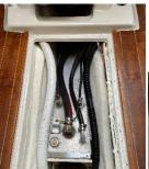
**Diesel Tank:** 19 Gallon Aluminum, vented overboard, no fuel cut off. (2) Hose appears solid, double clamped.
