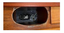
**Mast Support:** Keel stepped mast, through the table to a cast aluminum shoe fixed to the superstructure.
