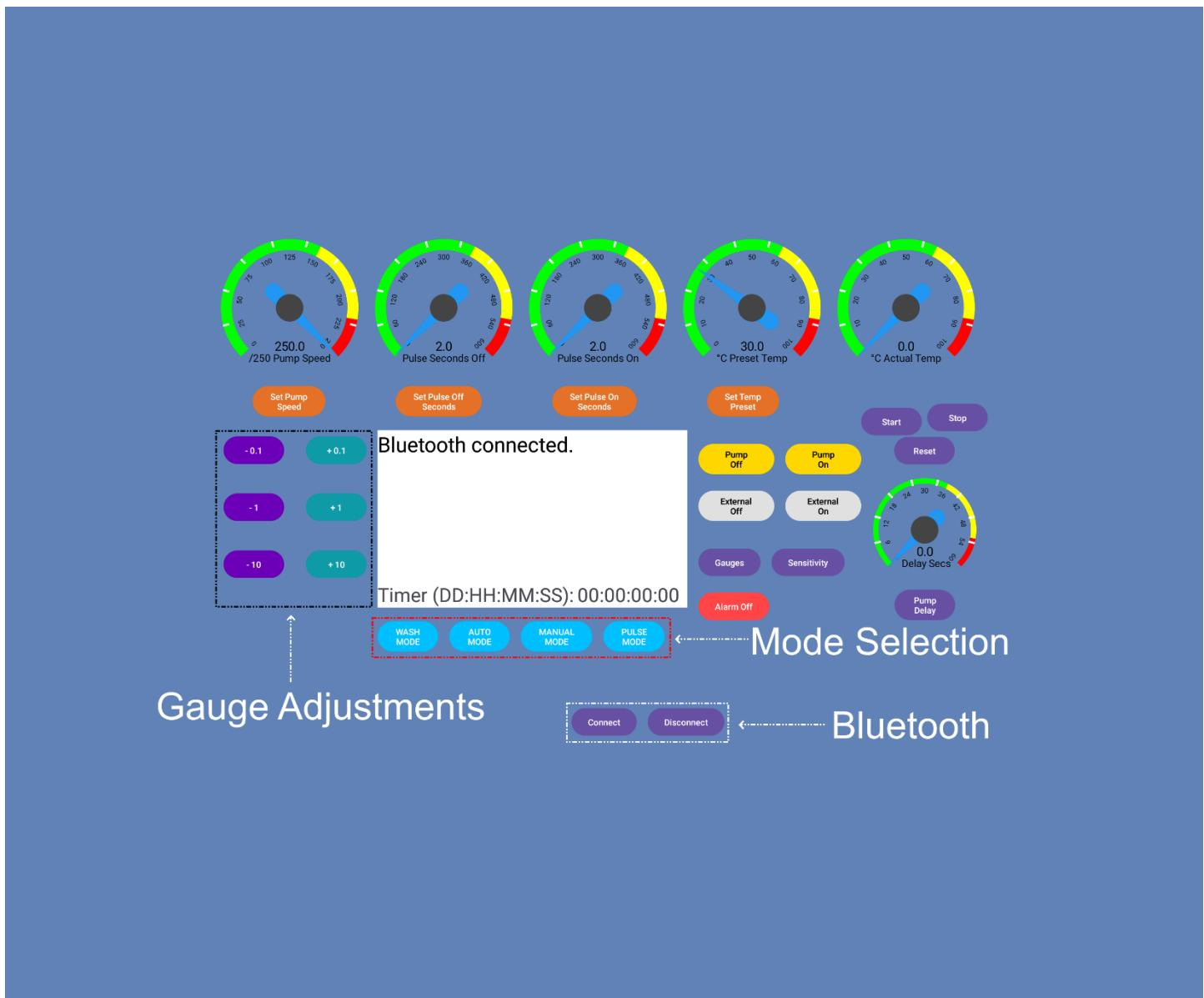
To adjust any gauge (except actual temperature), press the button under the gauge you require to change.
