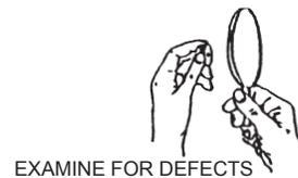
11. **NEVER** pull the JUICE BOX by its hose. Protect the hose from vehicular traffic and sharp objects. Be careful not to twist or kink the hose while the machine is in use. Do not use the hose if damaged. Do not use shut-off gun if there are any leaks from the packings or fittings.
