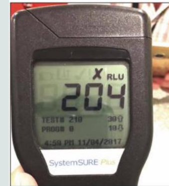
Baseline swab test of canteen table before application of Tersano Ozonated Water
