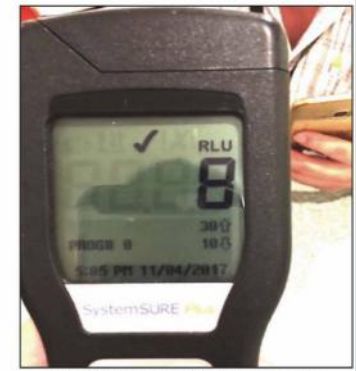
Bacterial count results after wiping the canteen table with a paper towel and Tersano Ozonated Water
