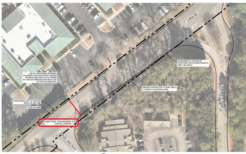
**ELECTRICAL ROUTING PLAN** SCALE: 1" = 40'
