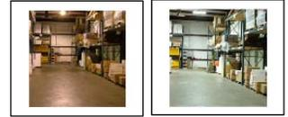
**Same design lumen can have different "usable light output" and "apparent brightness".**
