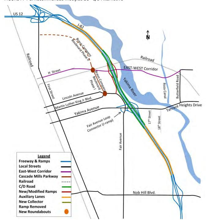
FIGURE PP4-1: Recommended Modified 2C - C/D Alternative
