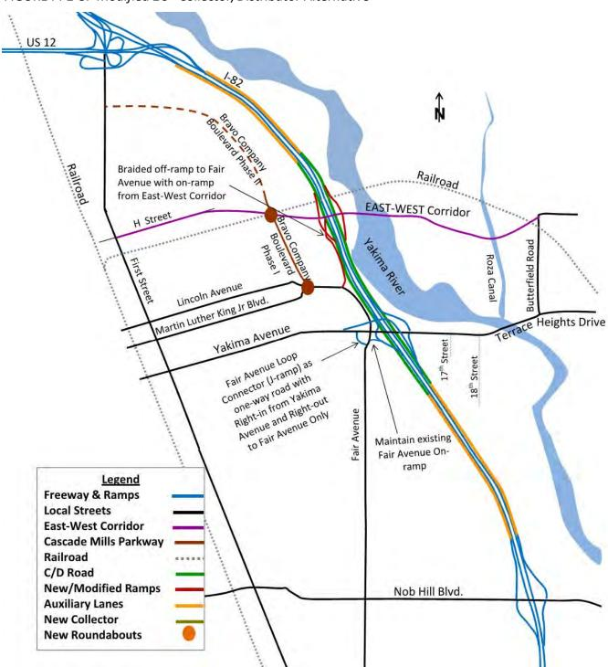
FIGURE PP2-8: Modified 2C - Collector/Distributor Alternative
