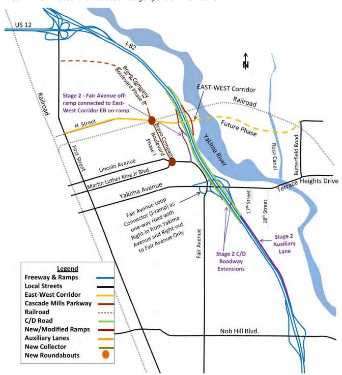
FIGURE PP3-11: Second Construction Stage of the CD Alternative
