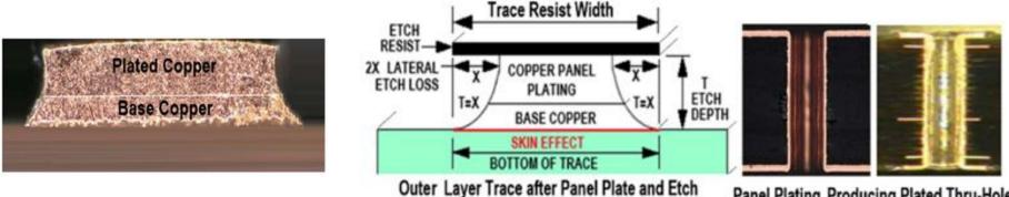
Panel Plating, Producing Plated Thru-Holes
