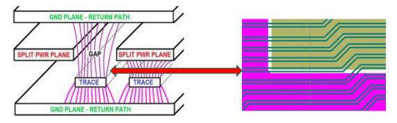
Routing Over *Split Gap* in PWR Planes will cause **Impedance Mis-match**
