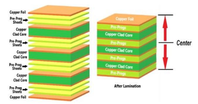
Bare Board 8-Layer Alternating Construction -Center Outward, Balanced on Both Sides
