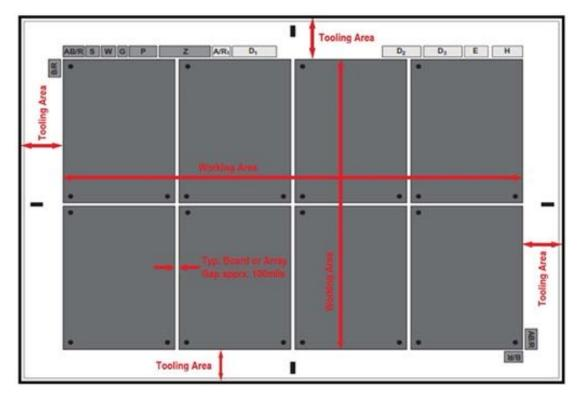
18" x 24" Fabrication Panel Sheet, Working Area and Tooling Area
