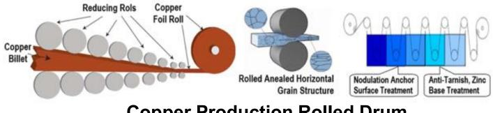
**Copper Production Rolled Drum, Pressed, and Surface Treatments**
