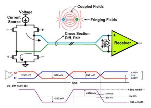
Pair of wires (Twisted pair) or two traces on a PWB, circuit **responds to electrical difference between two signals**, rather than difference between a single wire and GND, aka. single ended mode Any Impedance discontinuity caused by routing in a transmission line on one signal in the pair, can cause an SI issue and system failure
