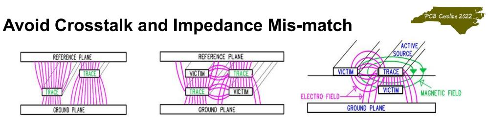
Planned vs. Actual, instead of two traces routed, 4 traces are routed. The actual routing did not equal the modeled topology,
