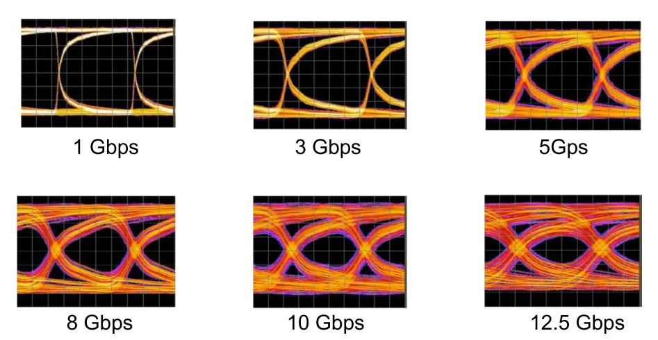
Using a lower loss material will open the "eye" at higher speeds.
