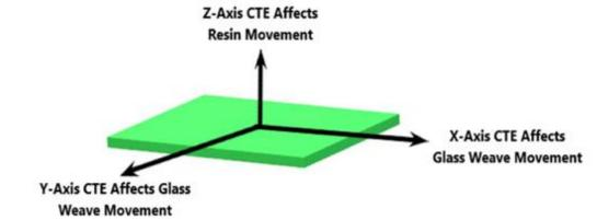
(CTE) Coefficient of Thermal Expansion in X/Y & Z Axis
