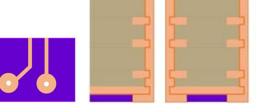
q. Resist-free area is plated with electrolytic copper
