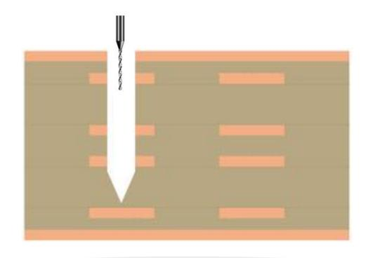
k. Drilling holes in laminated panel
