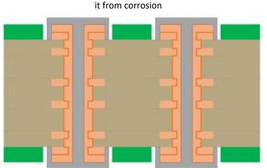
Final finish is applied to exposed copper to protect
