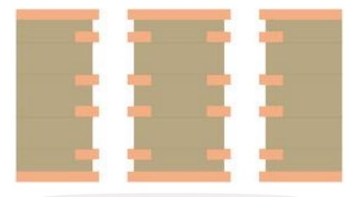
m. Cleaned and prepped holes, and etchback
