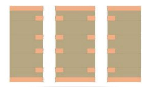
I. Resin smear in holes after drill process
