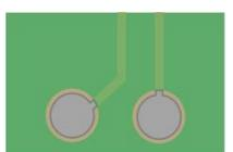
a. Final finish applied to exposed copper
