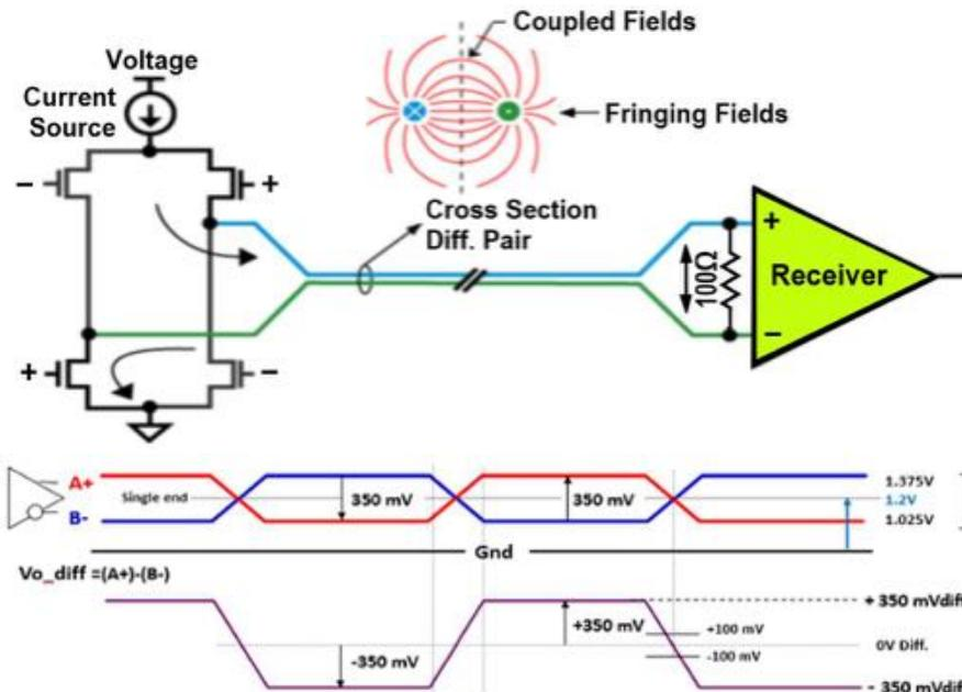
Any Impedance discontinuity caused by routing in a transmission line on one signal in the pair, can cause an SI issue and system failure
