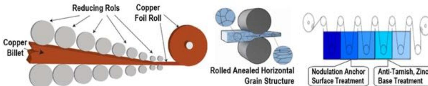
**Copper Production Rolled Drum, Pressed, and Surface Treatments**
