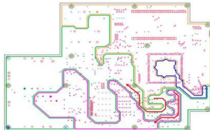
Routing Over *Split Gap* in PWR Planes will cause **Impedance Mis-match**
