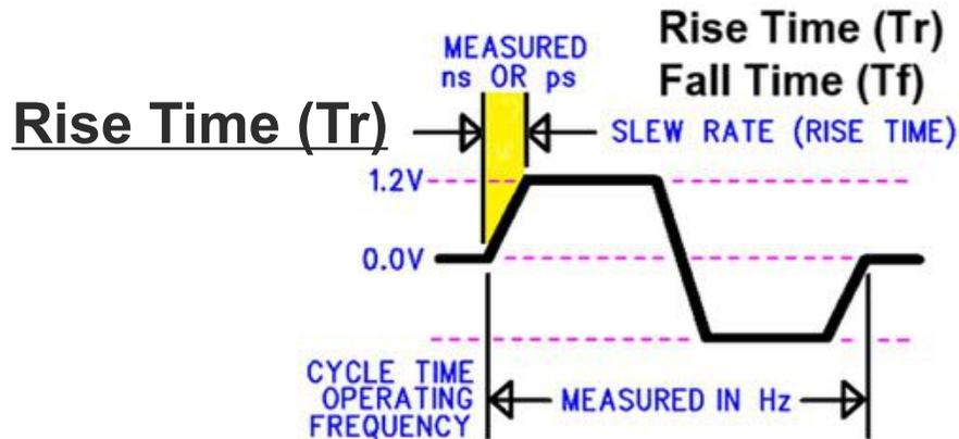
Trace length equal to  $\frac{1}{4}$  of the Rise Time (Tr) signal integrity issues such as reflections start to occur with any impedance discontinuities
