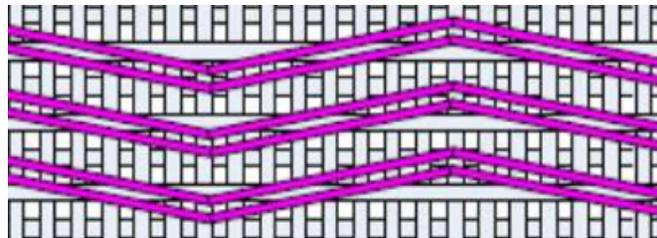
Fiber-weave Routing is an Inconsistent Solution
