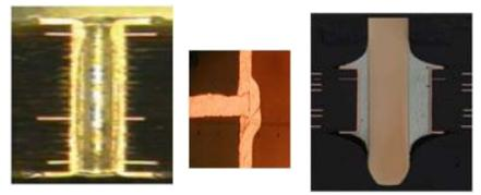
Plating step will inadvertently add an accumulated metal thickness to the layers at that step, whenever applied, will occur for every plated drill process and must be **accounted for when used across the entire panel, called panel plate**, or **selectively, called button plate**, where only holes are plated
