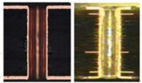
Panel Plating, Producing Plated Thru-Holes
