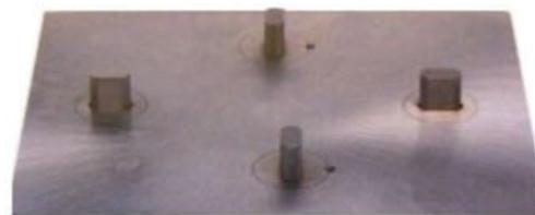
Lamination Base Plate with Pin Alignment
