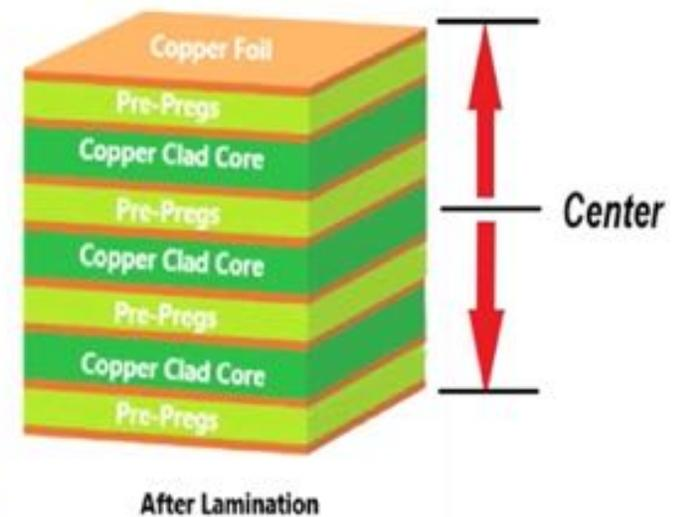
Bare Board 8-Layer Alternating Construction - Center Outward, Balanced on Both Sides
