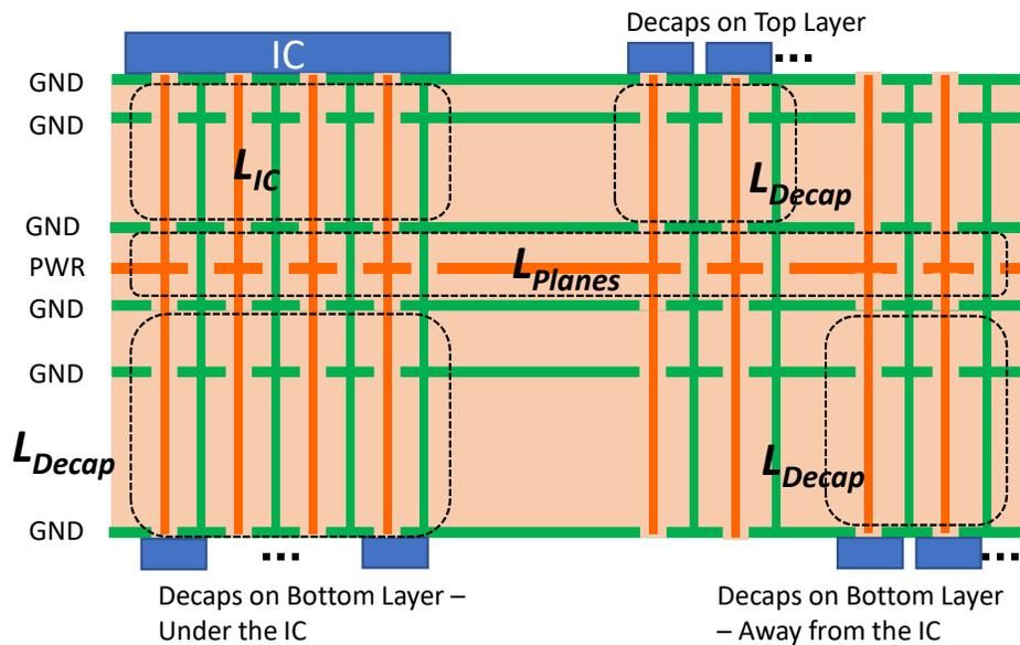
High-layer count PCB PDN geometry stack-up and  $L_{Decap}$ ,  $L_{IC}$  definition.
