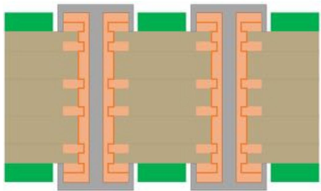
a. Final finish applied to exposed copper
