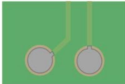
Final finish is applied to exposed copper to protect it from corrosion
