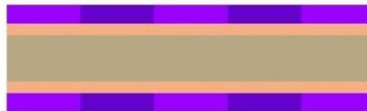
d. Polymerized pattern in resist
