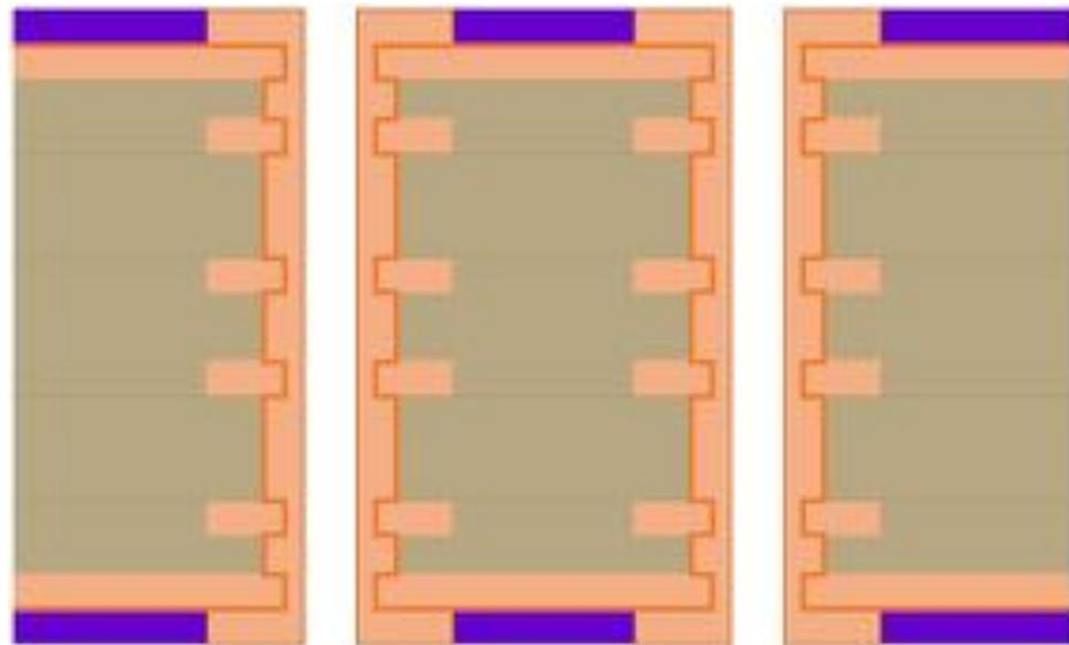
q. Resist-free area is plated with electrolytic copper
