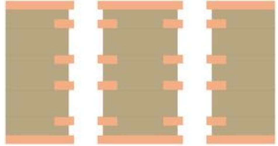
m. Cleaned and prepped holes, and etchback
