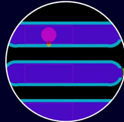
Pins too wide for pads can lead to insufficient side fillets of solder joints
