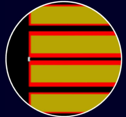
Gangmask is required for fine-pitch devices
