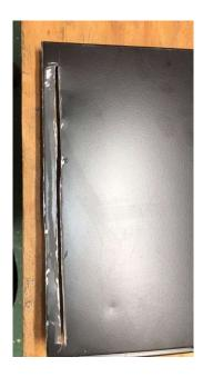
N. Remove the flange on the back upper left corner of the dedicated oven, circled in red below left (the photo shows a notch cut out of the flange, but the flange should be removed from the bottom of the notch shown all the way up, as indicated by the vertical red line).
