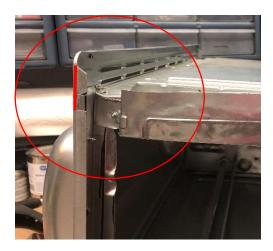
O. Remove the extensions of the dedicated oven sides that project above the top, cutting along the profile of the top (indicated by the two angular red cut lines below. Your oven will not yet have the opening depicted).
