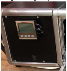
Your oven is now complete. Test the oven while monitoring it closely for any electrical issues and temperature. The extension box typically heats faster than the main oven, but both should hold a final temperature withing 5°f of each other.
