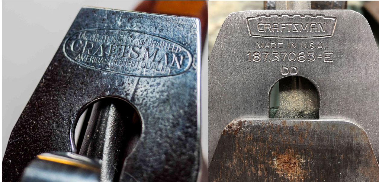
Figure 4 Sargent & Company keyhole up by trademark, left. Stanley Works keyhole down away from trademark with the 187-manufacturer code, right
