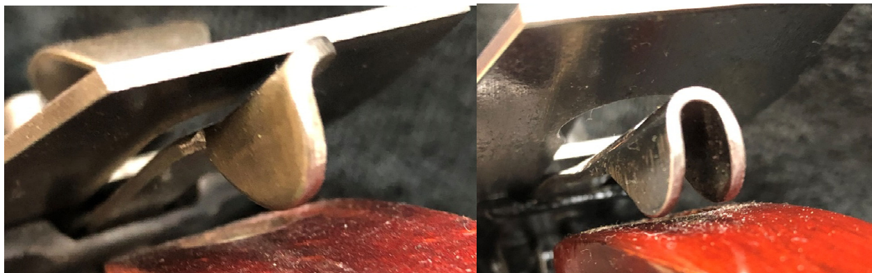
Figure 3 Millers Falls Tools left-hand bend lateral (left). Sargent & Company and Stanley Works inverted "U" lateral (right).
