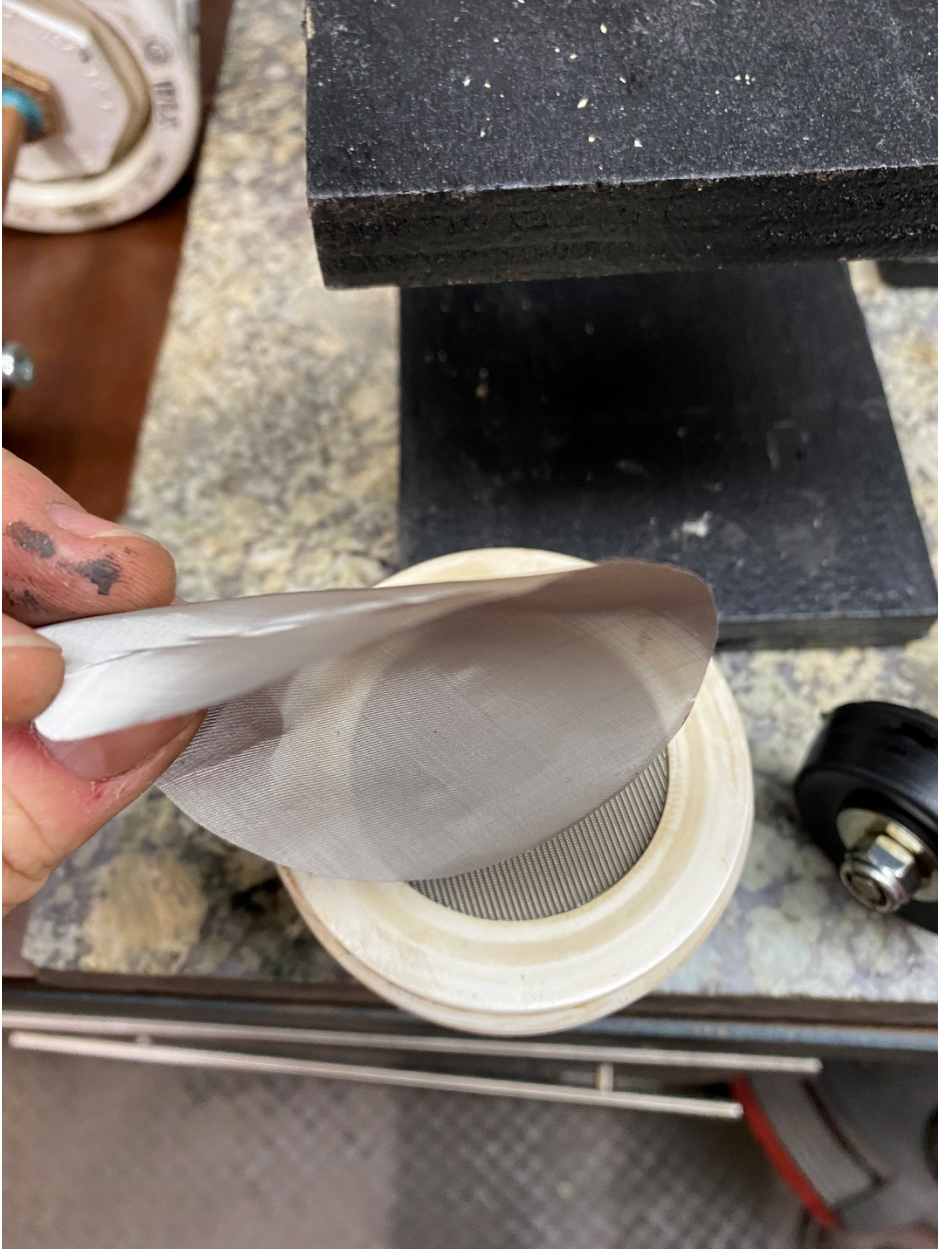
The fine filter media. Very flexible and must be supported. It is cut to also be held by the Union o-ring.
