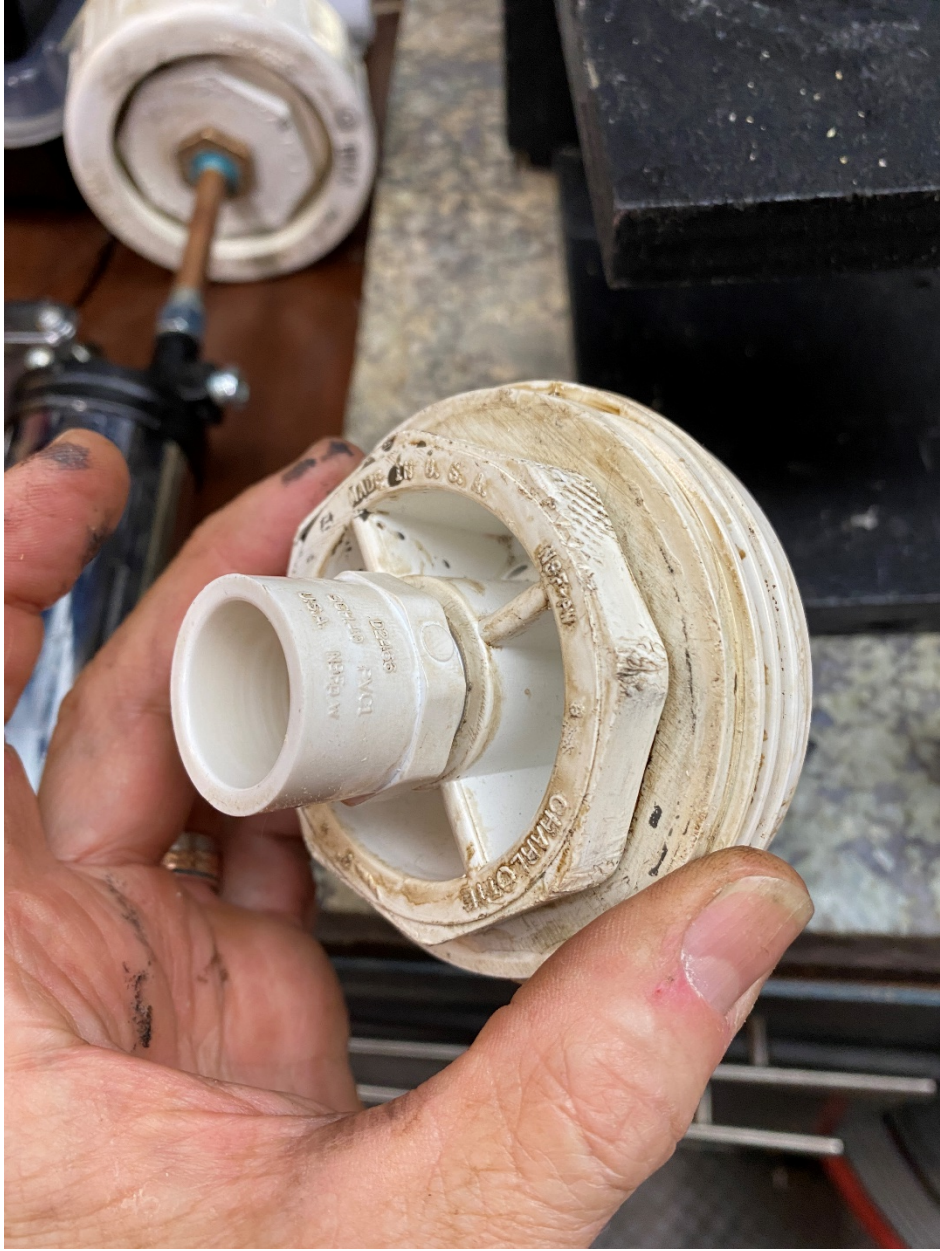
I added the 1/2" pvc fitting for an outlet spout to direct the filtered japanning into the small cans.
