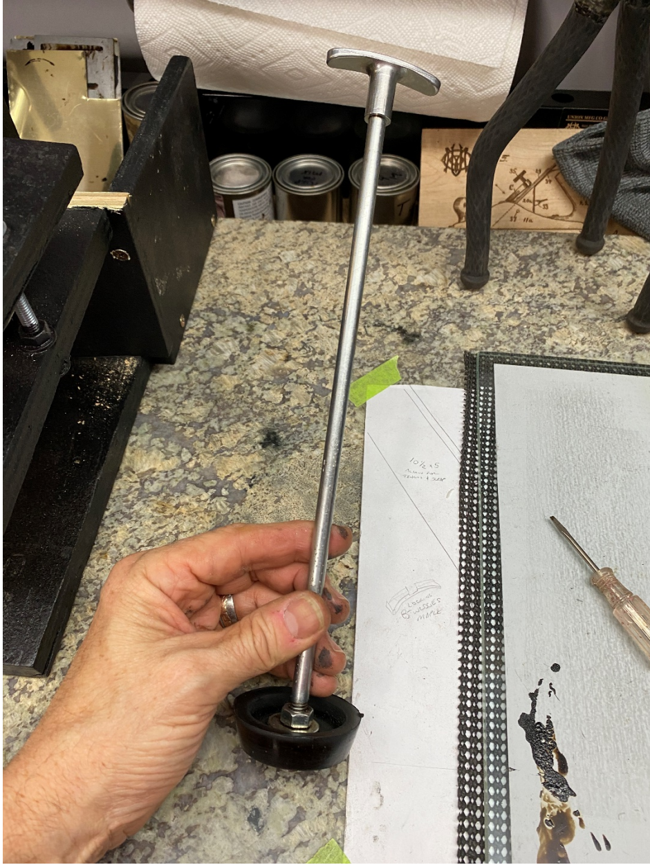
Added stopper nut to secure rubber plunger to rod.
