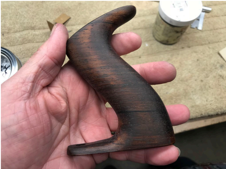
After removing AquaCoat and applying Goodfilla Ebony... wiping excess with damp cloth to prevent unwanted staining of the rosewood.
