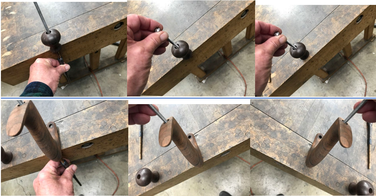
Showing dismount of totes and knobs when wet after spraying
