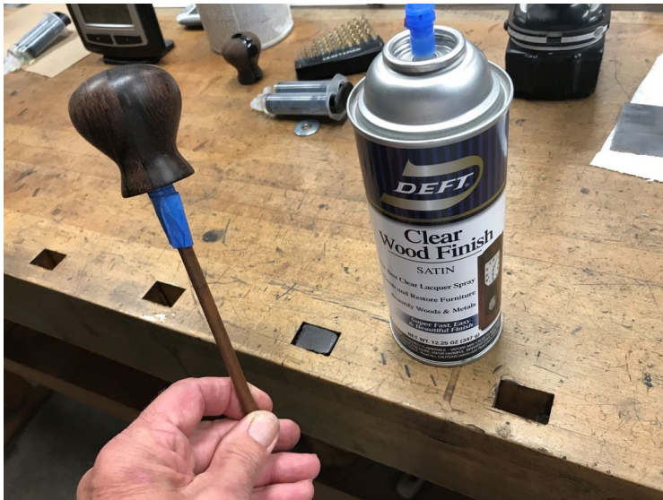
¼" dowel and blue tape to hold parts while spraying
