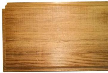
Thermally Modified Timber is achieved by using high temperatures in excess of 210 - 220°C (410 - 425°F). TMT have a distinctive chocolate brown colour all the way to the core due to the caramelization of sugars in the wood during the process. This results in products that are extremely durable no matter the environment in which they are used.
