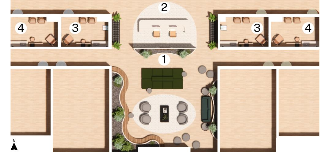
The floor plan arrangement is oriented to reduce solar gain and capture prevailing breezes, which allows for double the amount of **natural ventilation**.
