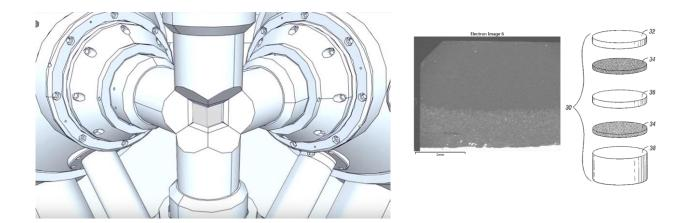
The XL Forced PDC cutter is the cutting-edge product used by PDT in challenging applications. Through a combination of multi diamond layers technology and diamond to carbide interface shape, this cutter has shown superior thermal resistance to rough solicitations providing enhanced bit life and drilling performances challenging any deep leached cutter.
