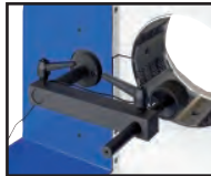
Back Limit Switch
