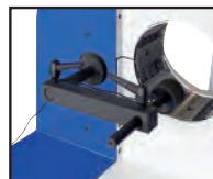
Back Limit Switch
