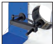
Back Limit Switch
