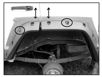
•Mark remaining holes through fender flares to sheet metal
