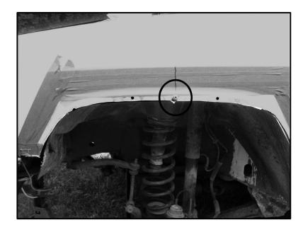
•Reattach center brace •Drill new hole if necessary
