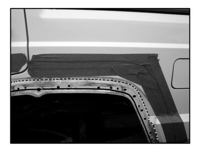
•Cut away the sheet metal below the spot welds. Do not remove the sheet metal with spot welds.
