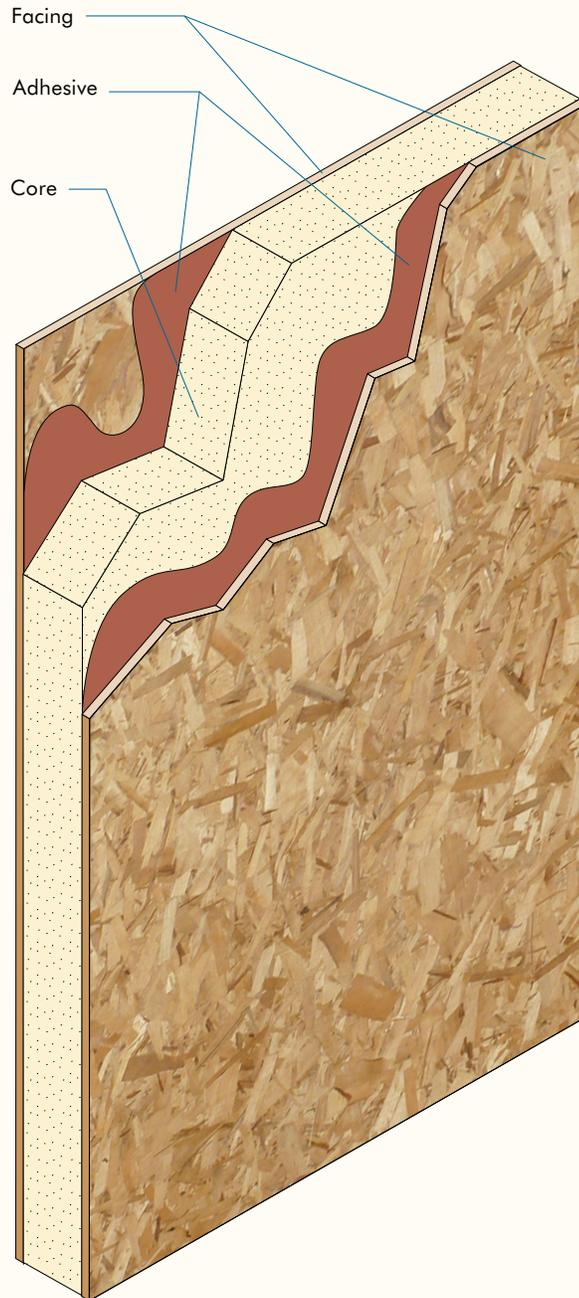
**Wood Structural Panel** – a panel product composed of oriented strand board (OSB) or plywood in conformance with the performance requirements of DOC PS1 or DOC PS2 in the U.S. or CSA O121, CSA O151, or CSA O325 in Canada, and the additional requirements specified in this standard
