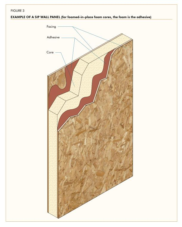
**Wood Structural Panel** – a panel product composed of oriented strand board (OSB) or plywood in conformance with the performance requirements of DOC PS1 or DOC PS2 in the U.S. or CSA O121, CSA O151, or CSA O325 in Canada, and the additional requirements specified in this standard
