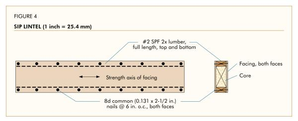
Edgewise bending tests shall be conducted in accordance with the third-point load method of ASTM D4761 with the additional requirement that the facings of the SIP specimens shall not bear on the supports of the test setup and the bearing length shall be 1-1/2 inches (38 mm). Load and deflection data shall be continuously recorded until failure.
