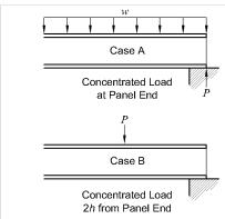
Figure 4.6.2.2: Bearing on Facings
