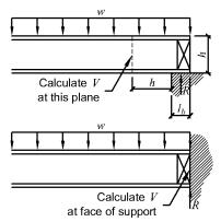
Figure 4.4.5: Design Shear Force
