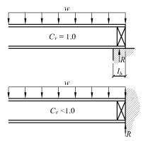
Figure 4.4.4: C<sub>V</sub> Support Conditions
