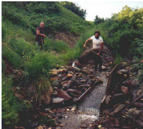
Above: Miners on Lucky Creek sluicing rusty gold. Home made wooden sluice.
