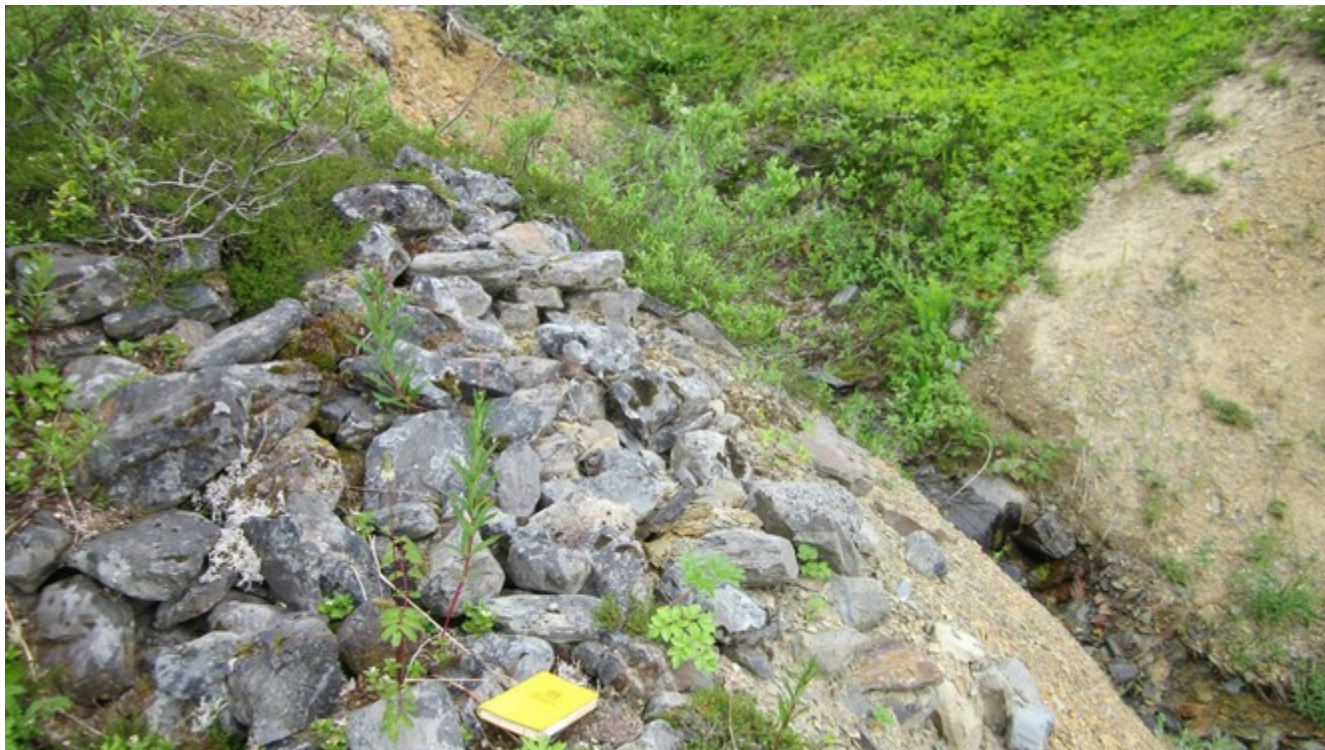
Image 1: Hand-stacked tailings and worked mining trench in gold-bearing Argillite, Potato Patch/Blue Ribbon Mine. Fieldbook is for scale. Bedrock, primarily Argillite is visible on the right. Free gold can be panned from this area. Large rocks are primarily Graywacke rolled down the mountain and thrown out of the pit and sluice.
