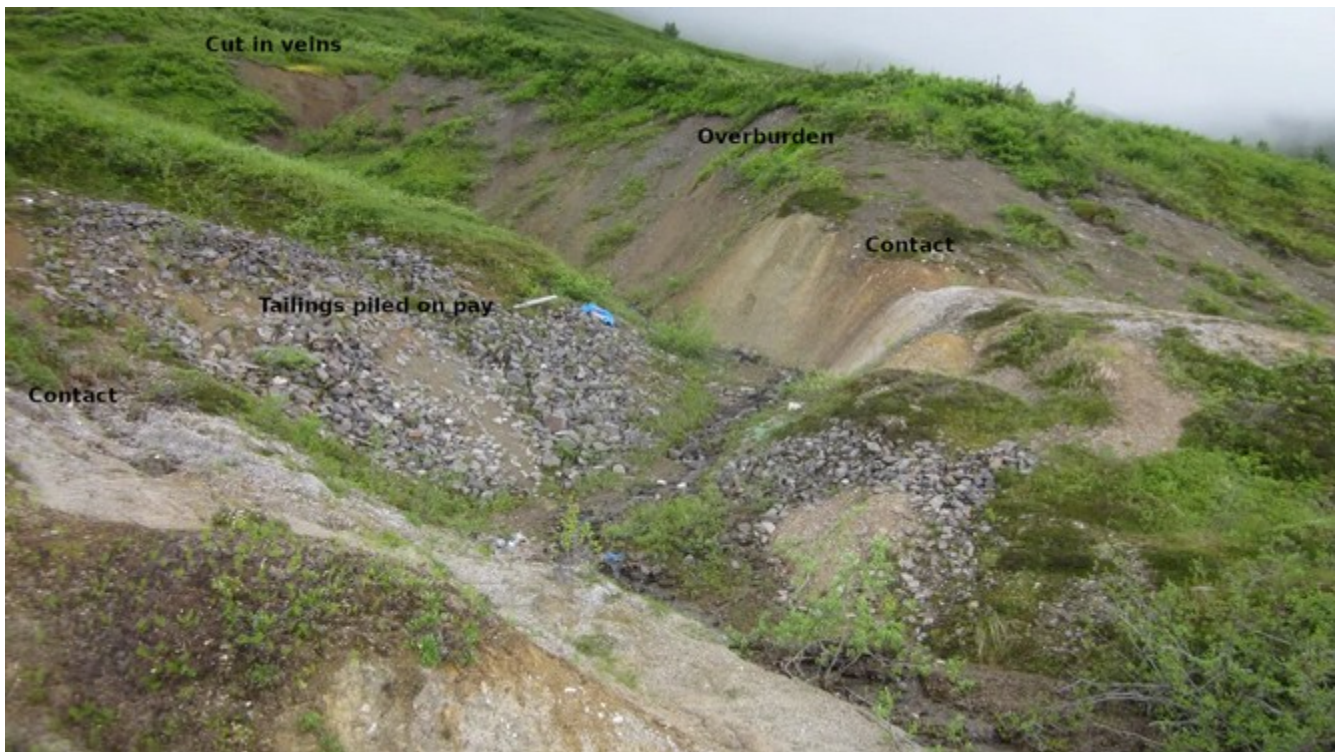
Fig. 3 View of The Potato Patch, showing contact, old mining pit, overburden, and cut in quartz veins.
