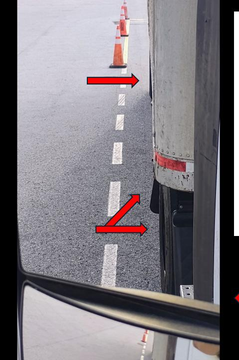
Check your mirrors often and if the trailer moves, move with it. The steering should be towards the problem, slow counter steers. Less trailer tire you see in the mirrors the straighter you are. Keep the corners behind the tractor drive tires and the drive tires underneath the trailer.
