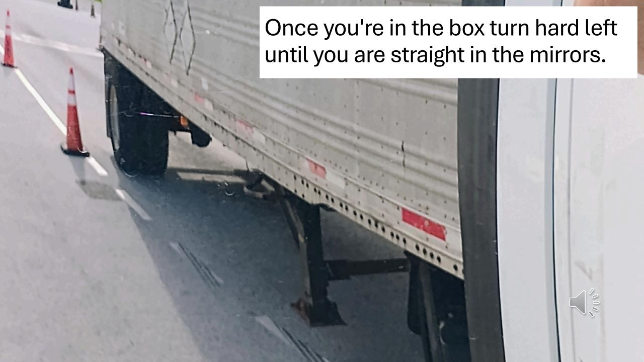
If you happen to come in a little bit crocked no worries just stop and pull up again, you have two free pull ups. Pull up and get straight in your mirrors, and in the box. Do not pass the last set of cones. Start to back up again.
