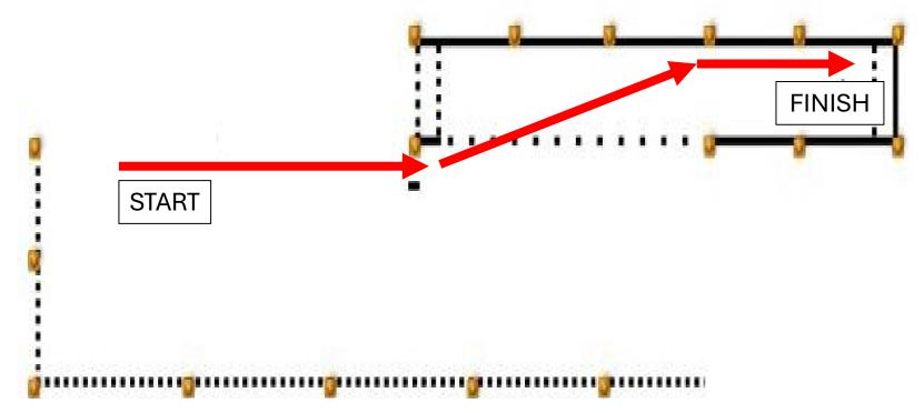
Starting parallel with the outer boundary, offset back into the alley, bringing the rear most part of your vehicle (other than unique vehicle parts higher than the door mirrors, such as a bucket truck) within three (3) feet of the rear of the alley. Stop with the rear most part of the vehicle (other than unique vehicle parts) in the three (3) foot box at the end of the alley.
