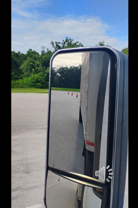
Start backing up and stay as straight as you can, while at the same time you aim just ahead of the 40-foot cone.
