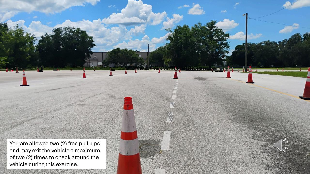
As you start backing up begin to turn the steering all the way, left to swing the trailer to the right, when you see the landing gear stop. Turn the steering all the way right. As the truck swings around stop when you are straight in your mirrors.
