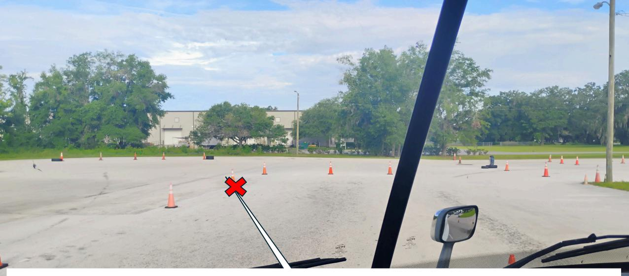
Pull forward to correct the angle by aiming at the second cone of the outside boundary. You will aim the front left part of your vehicle as if you are trying to run the cone over with the trailer tires.
