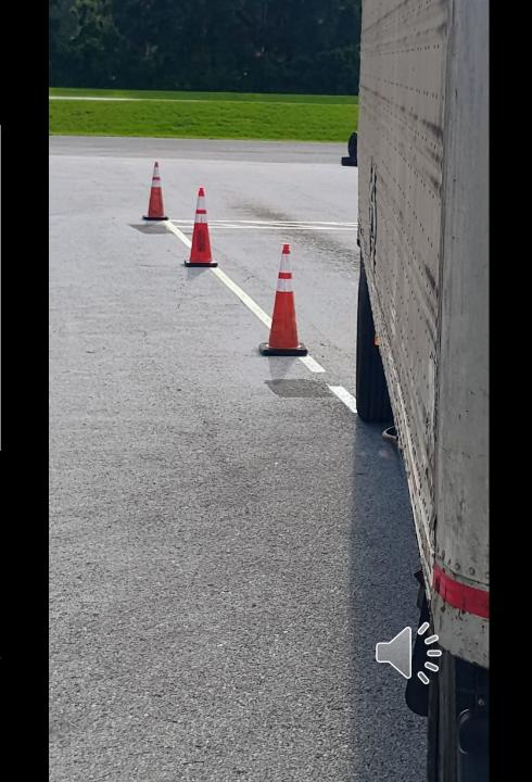
As you get closer to the 40-foot cone, once the trailer tire is split by the dotted line, turn hard right to push the trailer back into the box.
