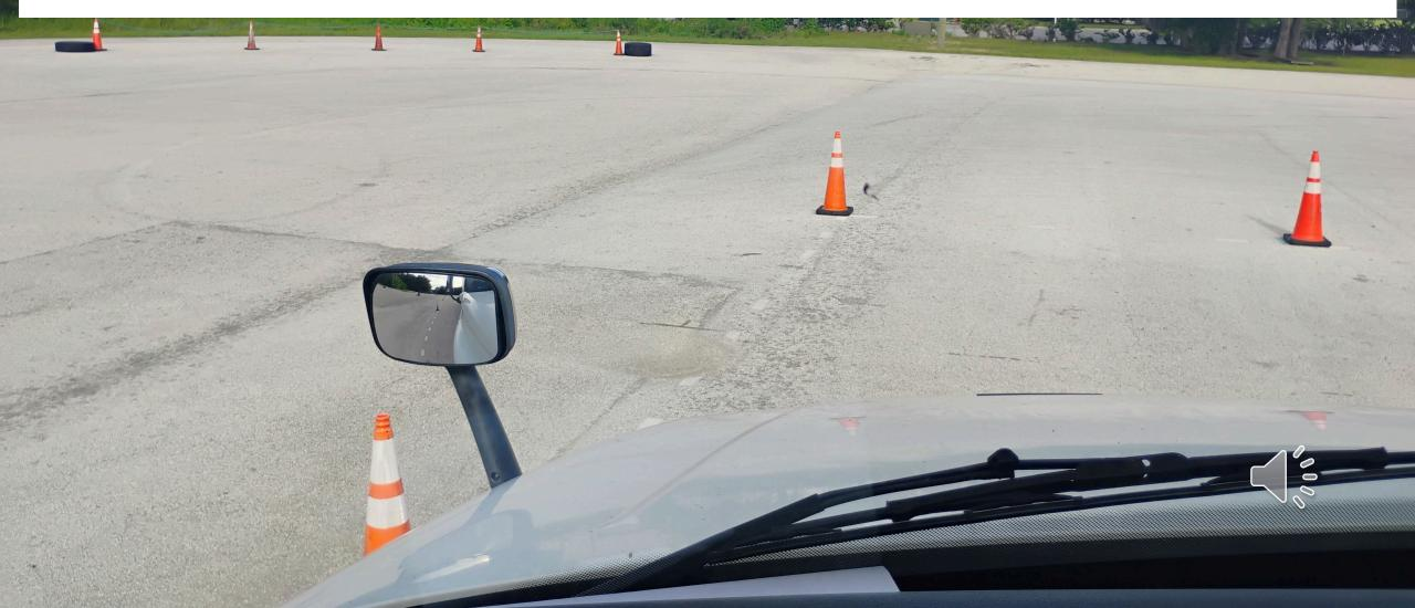
Start backing up and stay as straight as you can, while at the same time you aim just ahead of the 40-foot cone.
