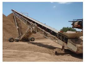
402 2001 Superior 36X125PS125 36"x125' Portable Radial Stacking Conveyor, 85,000 90,000 SN 4308, , hydraulic raise, power travel with hydraulic raise undercarriage, hydraulic folding end section, Weigh Shark belt scale, fifth wheel hitch. Good condition, good belt.
