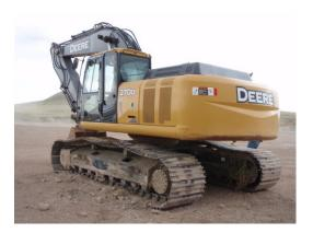
307 2011 John Deere 270D LC Hydraulic Excavator, SN 1FF270DXKA0704001, 120,000 163,500 ac cab, 12'4" stick, 52" bucket, 31.5" pads, auxiliary hydraulics, 2,706 hours. Very good condition, good undercarriage.
