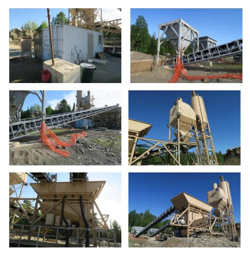
71-20-002 2001 Johnson-Ross Bandit 12 200 Cubic Yard Per Hour Portable Concrete Batch Plant, SN 68000, aggregate and cement storage, 12 yd aggregate batcher, 6 yd cement batcher, 42" x36' aggregate transfer conveyor with15 hp motor, air compressor, and water system mounted on tandem carrier; Johnson-Ross dust collector; 8'X16' feed hopper; 36"x100' lattice folding field conveyor; 8'x20' conex control house. Good condition. 130,000
