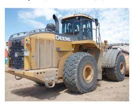
318 2012 John Deere 844K II Wheel Loader, SN 1DW844KXCCD644400, ac cab, gp bucket, ride control, Loadrite L2180 scale with ticket printer, rear camera, 29.5R25 tires, 5,533 hours. Good condition, good tires.
