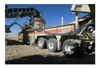
1999 Nordberg HP400SX Cone Crusher Plant, SN HP400226, 48" under cone discharge conveyor, twin 200 horsepower electric motors, hydraulic leveling legs, on tri-axle FabTec carrier, SN 2319799. Good condition.
