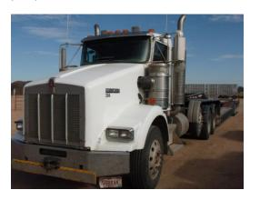
2042006 Kenworth T800B Tandem Truck Tractor, SN 1NKDLB0XX6R150752,<br/>Caterpillar C15 475 hp diesel engine, 18 speed transmission, engine brake,<br/>air lift 3 axle, 14,320 lb. front axle, 46,000 lb. rear axle, air ride suspension,<br/>356,162 miles. Good condition.57,50073,000
