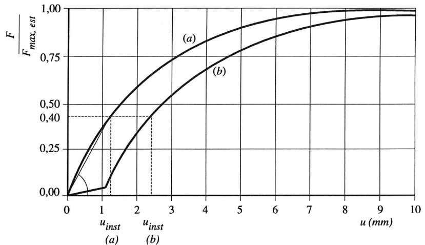
Figure 1 Idealised load-deformation curves of dowelled (a) and bolted (b) joints.
