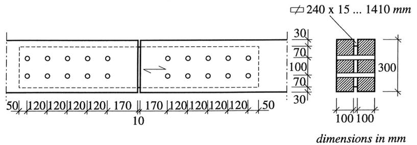
Figure 3 Dowelled joint with centre member of steel. Dimensions in (mm).
