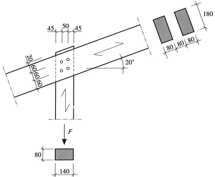
Figure 2 Double shear dowelled joint. Dimensions in (mm).
