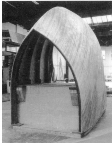
Figure 15 Structural model of a roof.
