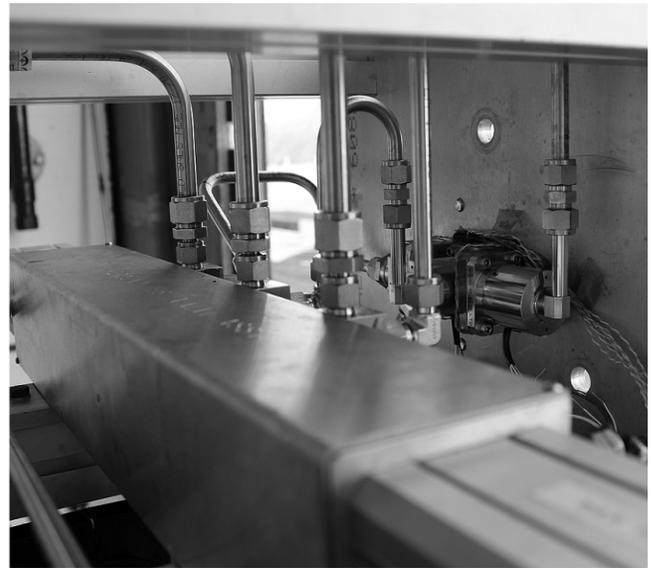
Fig. 6. A typical Development Model (DM) engine configuration mounted on the test stand at the Moog Westcott Operations sea-level hot-fire test facility. [Left] A view in front of the mounting plate showing a R512E/C103 workhorse combustion chamber with pressure taps and engine mounted thermocouples clearly visible. [Right] A view behind the mounting plate showing the DM valves connected to the engine.
