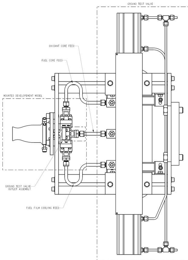
Fig. 5. A diagrammatic representation of a typical Development Model (DM) engine configuration mounted on the thrust stand. This is a top view of the horizontal-firing setup used throughout the test campaign. The propellant feed lines are connected to a Ground Test Valve (GTV) on the right. In the majority of the testing conducted, the static GTV Outlet Assemblies (GTVOA)'s shown on the engine were used in place of the DM valves.
