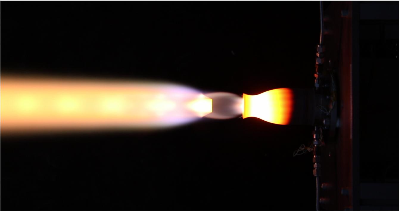
Fig. 7. An overhead optical camera view of a typical Phase 1B development model engine firing. The image shows one of the R512E/C103 workhorse chambers glowing at approximately 1400°C during testing at the Moog Westcott Operations sea-level hot-fire test facility.
