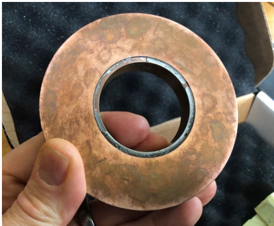
Figure 1: Compact electromagnet manufactured from high temperature superconducting material
